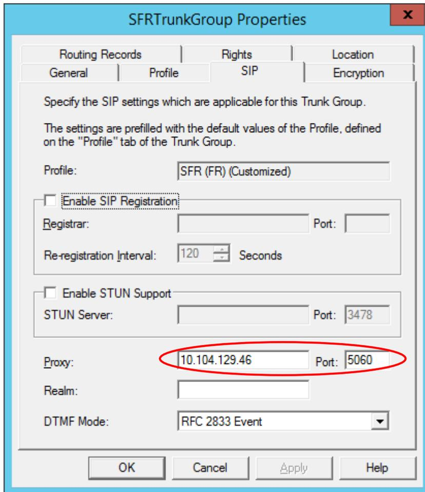
**Figure 21: The “SIP” tab of the properties dialog**
