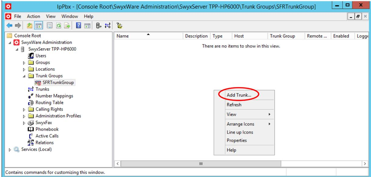
**Figure 22: Adding a SIP Trunk to the SIP Trunk Group**
